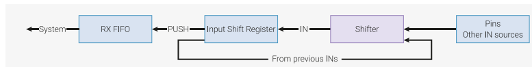
Figure 47. Input Shift Register (ISR). Data enters 1...32 bits at a time, and current contents is shifted left or right to make room. Once full, contents is written to the RX FIFO.
